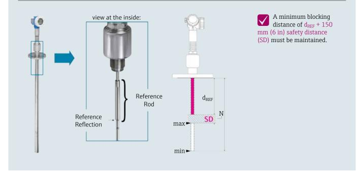
Figure 2: Gas Phase Compensation; Construction/Preconditions
