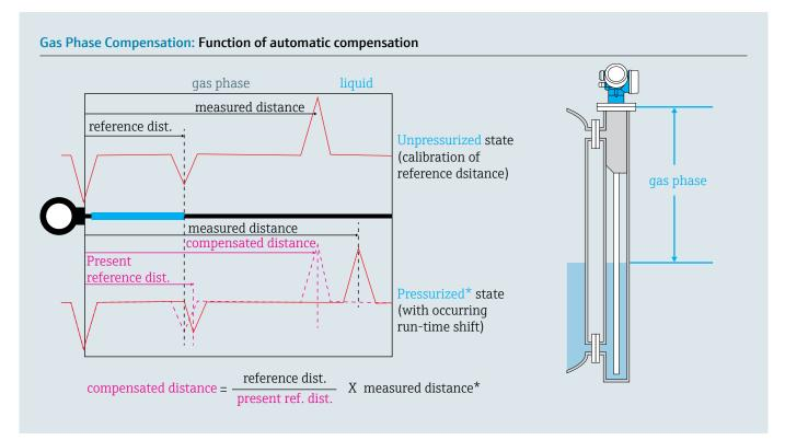
Figure 3: Gas Phase Compensation, function of automatic
