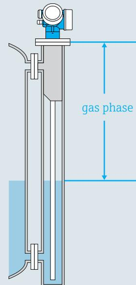
Figure 3: Gas Phase Compensation, function of automatic
