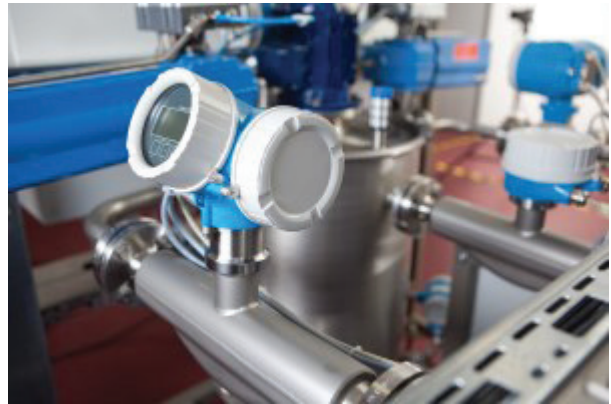
Figure 2: Flowmeters typically have to be removed from the process for calibration in a lab. On-board verification can determine when a flowmeter actually needs calibration
