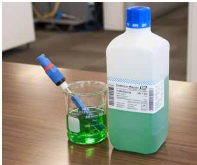
Figure 4: pH sensor being readied for calibration.
