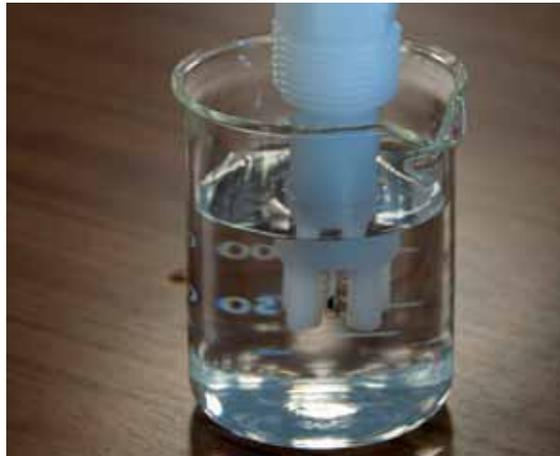
*Figure 2: pH sensor being kept wet in tap water.*
