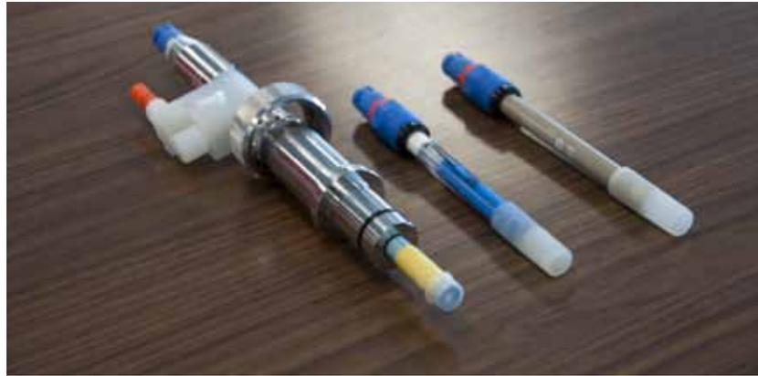
Figure 3: Store pH sensors with manufacturer's supplied boot/shipping cap or in beakers with storage solution.
