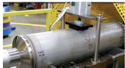
Promass I end connection welder Single straight tube design in five sizes, plus three full bore versions to optimize accuracy versus pressure drop. Coriolis flow tubes are constructed of 904L, 316L, Alloy C22, titanium or zirconium
