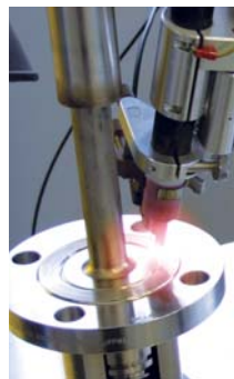
TIG Welding system Level and pressure instruments may be subjected to extreme conditions, each step in their manufacture has to lead to the highest quality product
