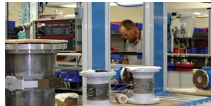
Magmeter assembly Different liner materials are required, depending upon the application. Liner materials range from PTFE, PFA, polyurethane, hard rubber, soft rubber and natural rubber
