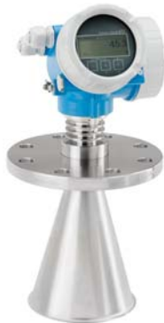
Figure 3: A radar instrument sends a microwave to the surface of a liquid or solid, and measures the time of flight for the reflected signal to determine level.
