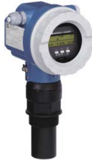
Figure 2: An ultrasonic sensor sends a sonic pulse to the surface of a liquid or solid, and measures the time of flight for the reflected signal to determine level.
