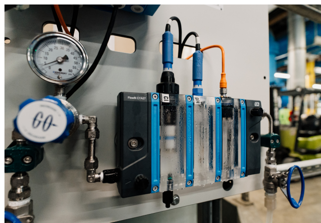
Digital total chlorine sensor Memosens CCS53E (left), digital pH sensor Memosens CPS11E and Flowfit CYA27 assembly
