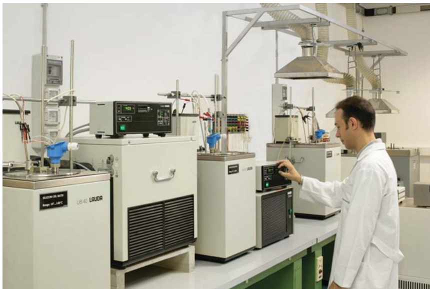
Figure 6: This Endress+Hauser lab can calibrate a sensor and transmitter, or determine CVD constants for an RTD and probe.
