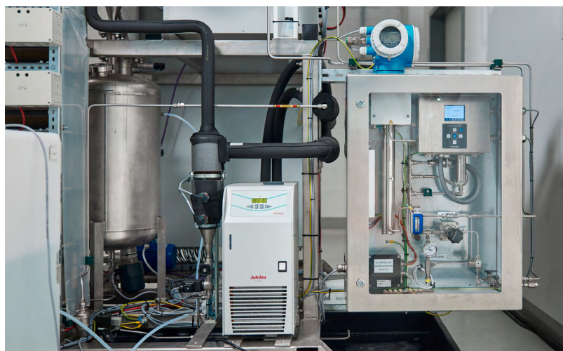
Measurement solution to test the process in an anion exchange membrane (AEM) electrolyzer.
