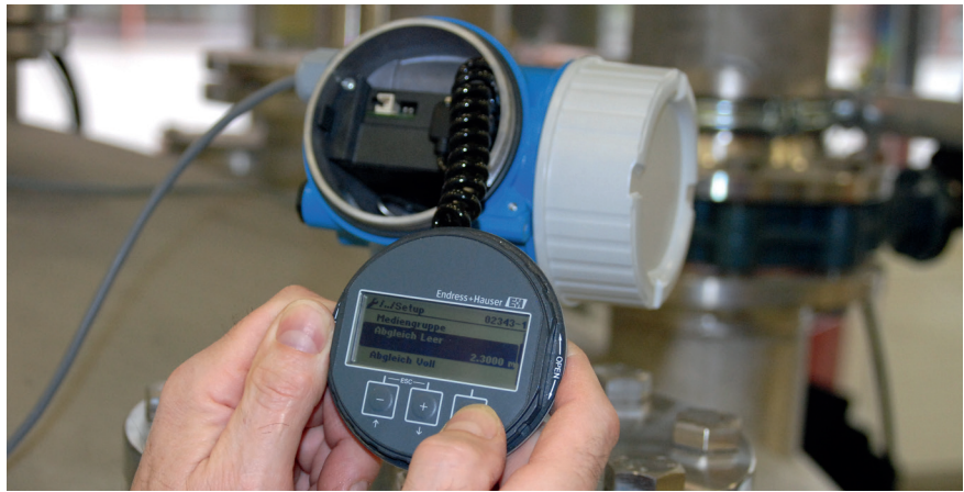
FIGURE 6. The display of an Endress+Hauser radar instrument stores all the instrument's parameters and transfers them to a replacement unit, simplifying maintenance and commissioning.
