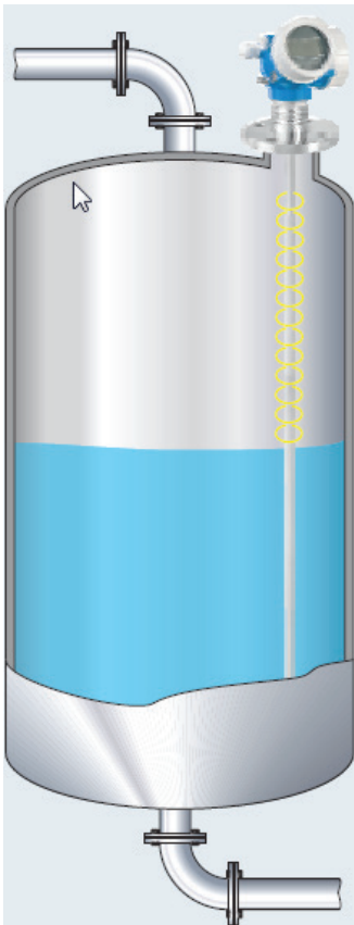
Figure 2: A guided wave radar transmitter sends a microwave pulse that reflects off the surface of the material. The time it takes for the pulse to return determines the level
