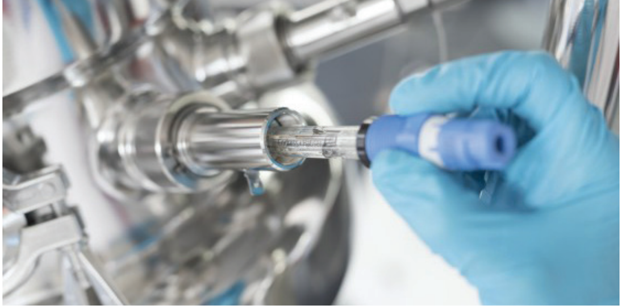
Figure 4: The Endress+Hauser CPS171D pH sensor has a glass membrane and reference gel that withstands SIP and CIP procedures
