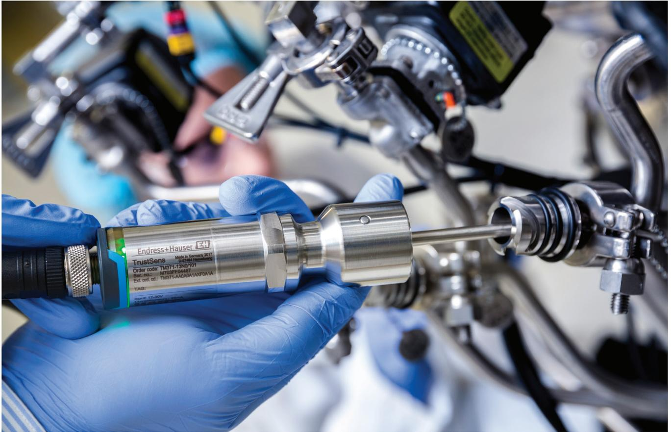
**Figure 5:** The Endress+Hauser TrustSens is a self-calibrating RTD sensor. It self-calibrates during every SIP procedure.
