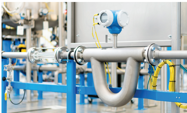
Figure 1: The Endress+Hauser Promass Q Coriolis flowmeter has a petroleum package that not only measures flow, density and temperature, it provides Net Oil, API gross and net volume calculations, viscosity and Reynolds number trending
