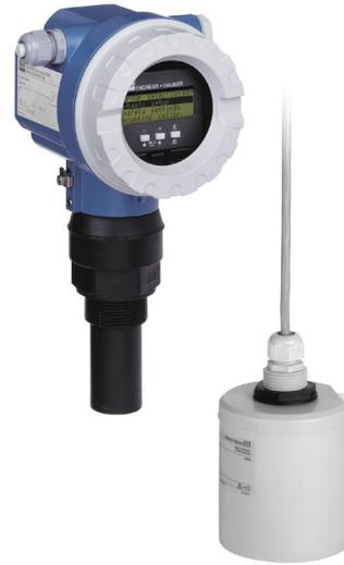
Figure 3: An ultrasonic sensor sends a sonic pulse to the surface of solids in a silo, and measures the time of flight for the reflected signal to determine level
