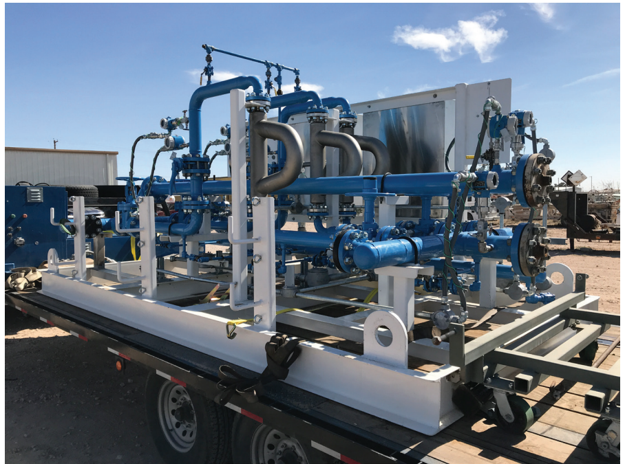
Figure 4: The Endress+Hauser HP80 Field Reference Meter Standard mounted on a trailer brings the capabilities of a calibration lab to the shale field.
