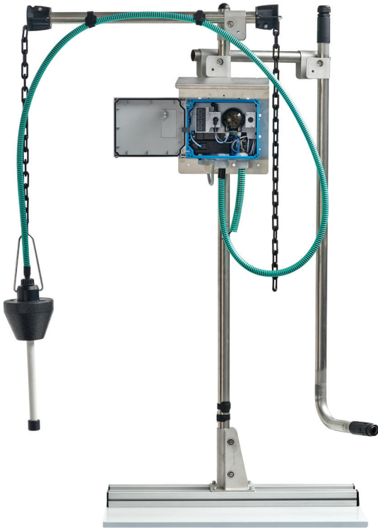
Figure 2: A sample preparation system, such as this Endress+Hauser CAT820, filters and delivers a sample to the colorimetric analyzer.
