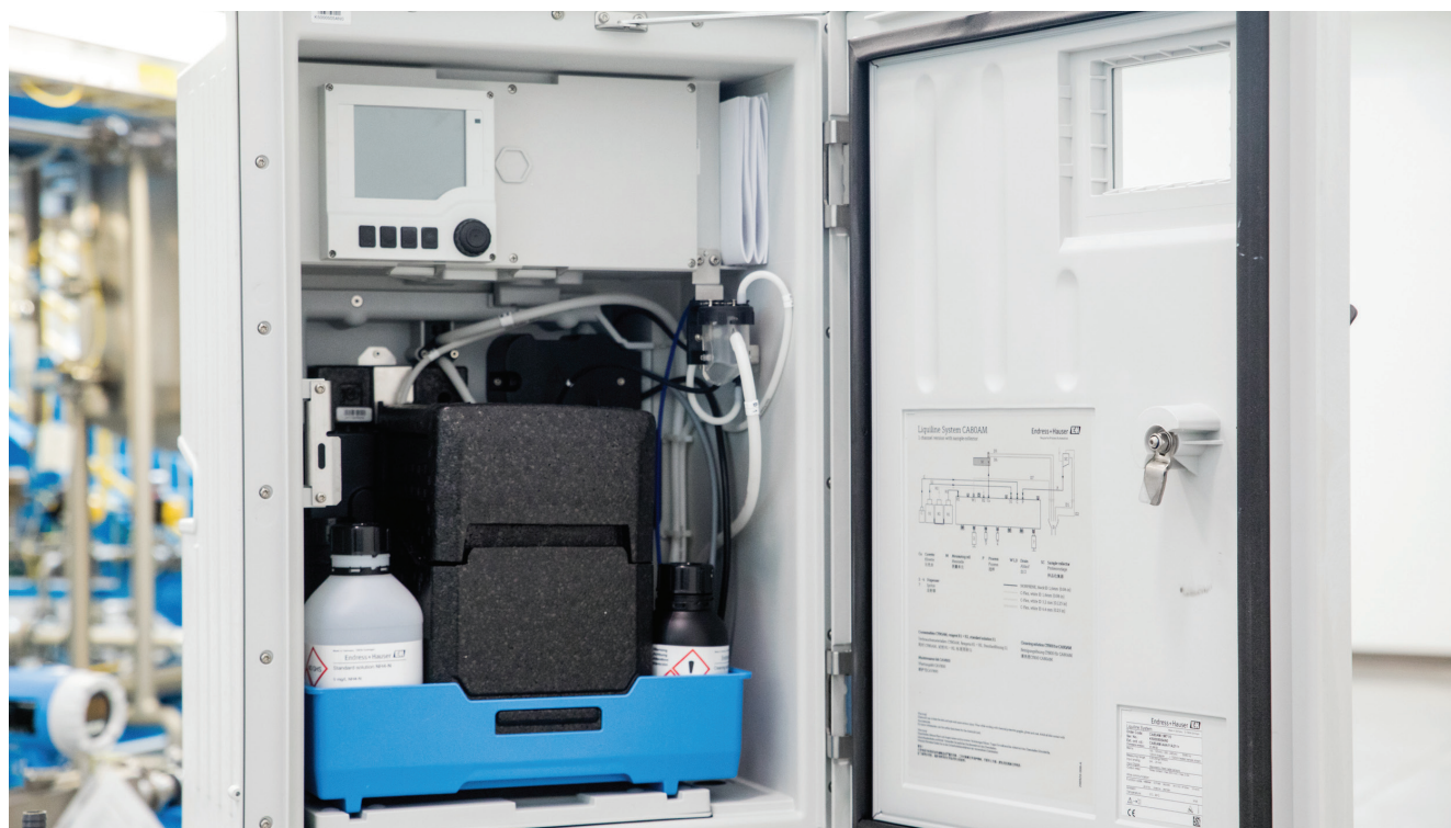
Figure 1: Ammonium or orthophosphate can be measured using photometric/colorimetric analyzers. Shown is an Endress+Hauser CA80PH orthophosphate analyzer.
