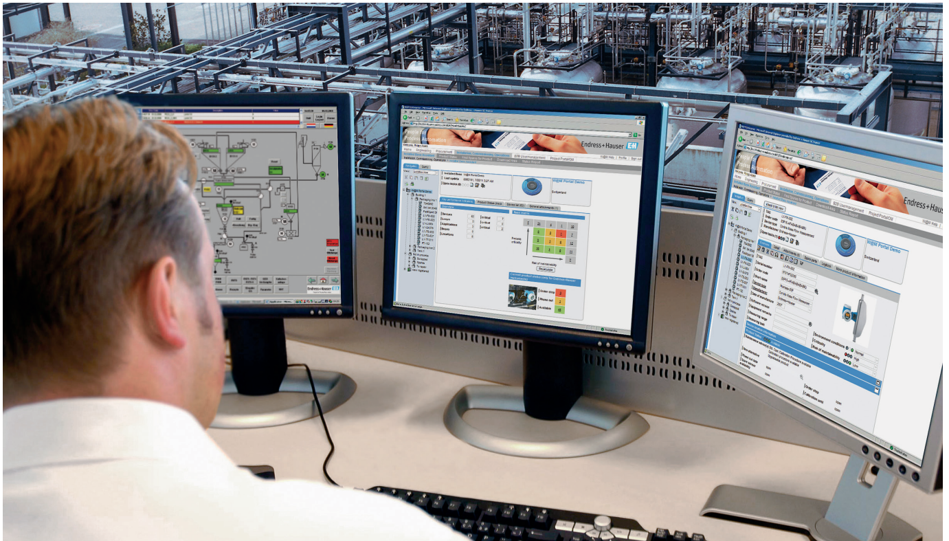
Figure 3: Instrument data from asset management software such as Endress+Hauser's W@M program can be accessed from workstations or handheld devices.
