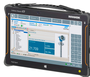
Figure 2: Asset management programs provide equipment manuals, parts lists and other information to handheld devices, such as Endress+Hauser's Field Xpert SMT70.
