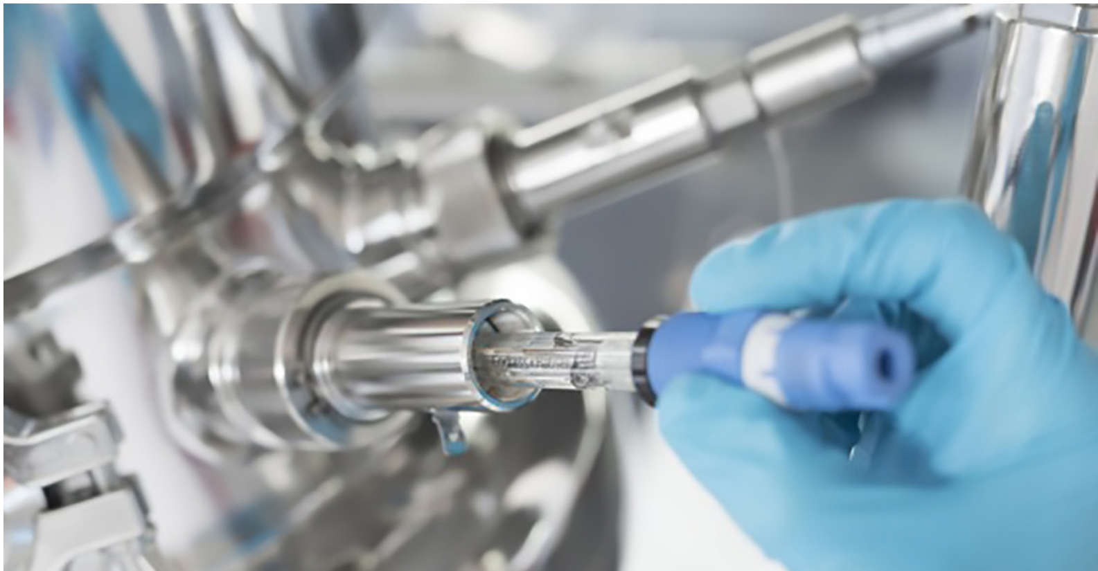
Figure 4: The Endress+Hauser CPS171D pH sensor has a glass membrane and reference gel that withstands SIP and CIP procedures
