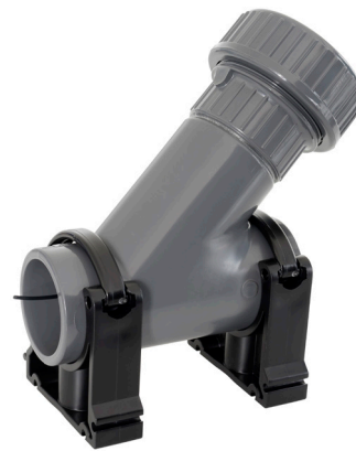
Figure 2: Y Strainer Provides “inertial filtration” of larger solids while allowing a representative process sample to enter the analyzer for digestion and analysis for an accurate, online, total phosphorus analysis. Automatically back washed before every measurement cycle and manually cleaned only when necessary (when a dosing fault is detected).
