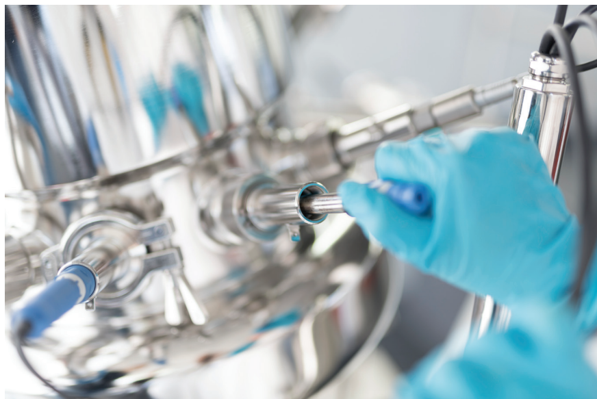
FIGURE 1. Digital sensors, such as these pH and conductivity probes in a fermenter production process, make it possible to use the same sensor in a process development lab, pilot plant and production process, thus simplifying scale-up.
