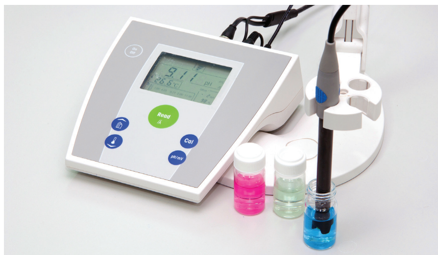
FIGURE 3. Analog pH sensor calibration system.
