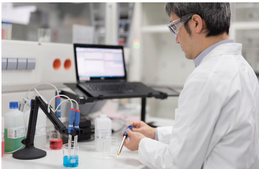
FIGURE 2. The same pH sensor used for a fermentation process can also be used in R&D and the process plant's lab.
