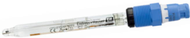
Figure 5: Endress+Hauser's CPS171D pH sensor stores measuring and operating data in the sensor including serial number, calibration date, number of calibrations, offsets, pH application range, number of calibrations, hours of operation under extreme conditions and other information.
