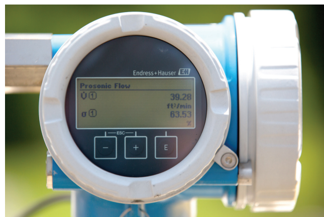
Figure 2: In the past, measuring the flow and methane content of biogas was difficult and expensive. Ultrasonic flowmeters proved to be a better solution.
