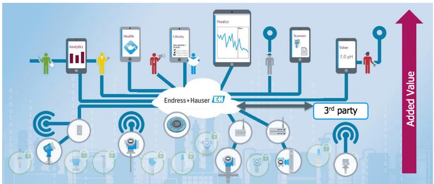
Figure 5: Cloud-based systems can off-load platform hosting, but also support asset health monitoring as a service, such as Endress+Hauser's Netilion Health.
