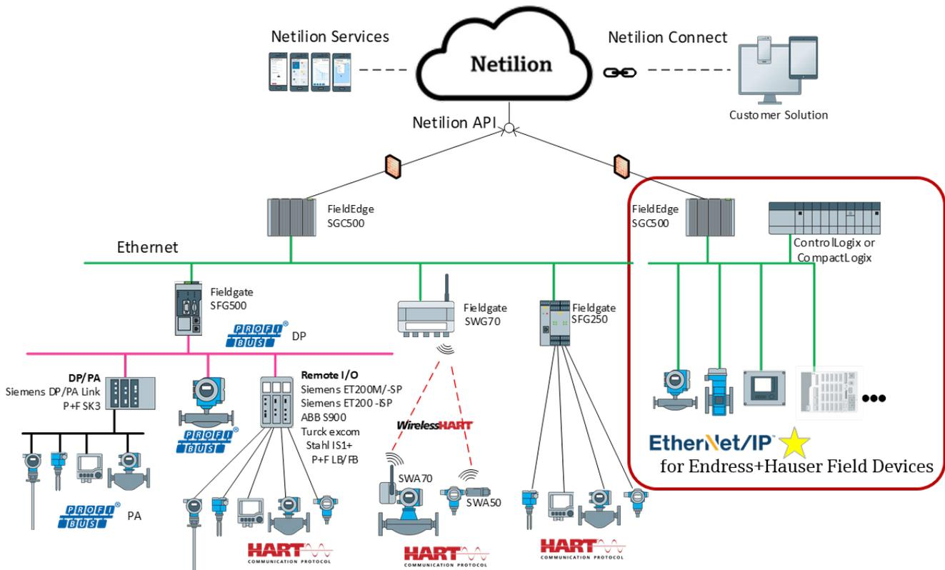
**Figure 3:** Industrial Internet of Things (IIoT) and Industry 4.0 examples are available now for learning how to apply in the field at a PTU.
