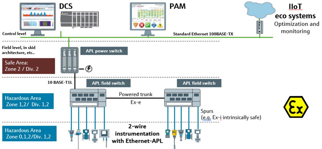
Figure 4: New IEEE 802.3cg standard and the next generation of plant networking and communications, such as the Ethernet Advanced Physical Layer, will be on full display at training facilities for hands-on learning at a PTU.
