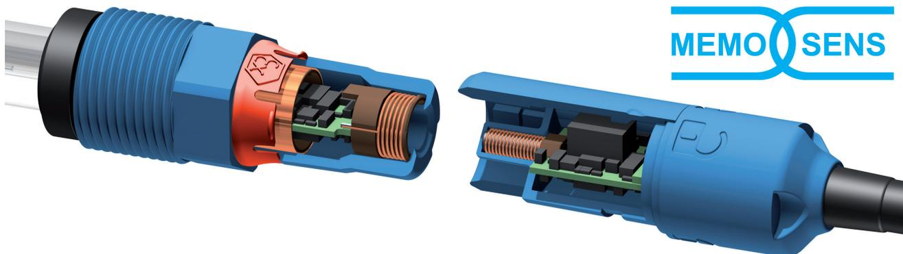
Using inductive coupling – for power and bidirectional data transmission – the galvanically isolated Memosens digital sensors tackle the major problems associated with pH measurements at their roots such as moisture and corrosion.
