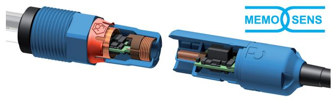
Using inductive coupling – for power and bidirectional data transmission – the galvanically isolated Memosens digital sensors tackle the major problems associated with pH measurements at their roots such as moisture and corrosion.
