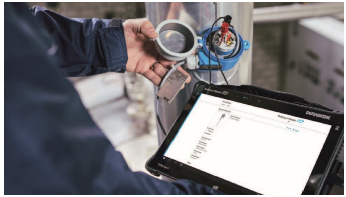
Figure 4: The Endress+Hauser SMT70 Field Xpert configurator tablet creates a mobile workstation in the field, and it can even be used in hazardous areas, enabling Heartbeat Technology and other diagnostic work without interrupting a process.
